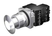
30mm Command/52, Chrome Finish Heavy Duty,Watertight/Oiltight Complete Metal Unit Illuminated Push-Pull Operator Transformer type, 600V AC LED Lamp Mushroom Head Cap Small 1 3/4" (44.5 mm) Metal, Chrome with White Lens 3 Position Momentary 1 N.C.+1 N.C. Extra Late Break Heavy Duty Contacts, A600/P600 UL Listed, CSA Certified NEMA 1,3,3R,4,4X,12,13 & Automotive Standards
