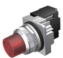
30mm Command/52, Chrome Finish Heavy Duty,Watertight/Oiltight Complete Metal Unit Illuminated Indicator Light Transformer type, 600V AC Super Bright LED Lamp, BA9s Glass Lens, Red UL Listed, CSA Certified NEMA 1,3,3R,4,4X,12,13 & Automotive Standards
