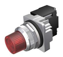
30mm Command/52, Chrome Finish Heavy Duty, Watertight/Oiltight Complete Metal Unit Illuminated Indicator Light Transformer type, 600V AC LED Lamp, BA9s Glass Lens, Red UL Listed, CSA Certified NEMA 1,3,3R,4,4X,12,13 & Automotive Standards
