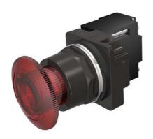
30mm BlackMax, Epoxy Coated Corrosion Resistant Metal Operator, Round Illuminated Twist-to-Release Full Voltage, 24V AC/DC Incandescent Lamp Mushroom Head Cap Small 1.79" (45 mm) Plastic Cap, Red 2 Position Maintained, Twist-to-Release UL Listed, CSA Certified NEMA 1,3,3R,4,4X,12,13 & Automotive Standards
