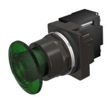
30mm BlackMax, Epoxy Coated Corrosion Resistant Metal Operator, Round Illuminated Twist-to-Release Full Voltage, 6V AC/DC Incandescent Lamp Mushroom Head Cap Small 1.79" (45 mm) Plastic Cap, Green 2 Position Maintained, Twist-to-Release UL Listed, CSA Certified NEMA 1,3,3R,4,4X,12,13 & Automotive Standards
