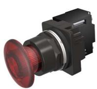
30mm BlackMax, Epoxy Coated Corrosion Resistant Complete Metal Unit Illuminated Push-Pull Operator Full Voltage, 24V AC/DC Incandescent Lamp Mushroom Head Cap Small 1 3/4" (44.5 mm) Plastic, Red 2 Position Maintained, Pull-to-Release UL Listed, CSA Certified NEMA 1,3,3R,4,4X,12,13 & Automotive Standards
