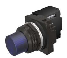
30mm BlackMax, Epoxy Coated Corrosion Resistant Complete Metal Unit Illuminated Indicator Light Transformer type, 240V AC LED Lamp, BA9s Glass Lens, Blue UL Listed, CSA Certified NEMA 1,3,3R,4,4X,12,13 & Automotive Standards
