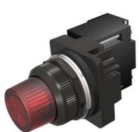
30mm BlackMax, Epoxy Coated Corrosion Resistant Complete Metal Unit Illuminated Indicator Light Full Voltage type, 120V AC/DC Incandescent Lamp, BA9s Glass Lens, Red UL Listed, CSA Certified NEMA 1,3,3R,4,4X,12,13 & Automotive Standards
