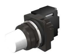
30mm BlackMax, Epoxy Coated Corrosion Resistant Complete Metal Unit Illuminated Indicator Light Full Voltage type, 12V AC/DC Incandescent Lamp, BA9s Glass Lens, White UL Listed, CSA Certified NEMA 1,3,3R,4,4X,12,13 & Automotive Standards
