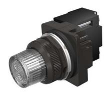
30mm BlackMax, Epoxy Coated Corrosion Resistant Complete Metal Unit Illuminated Indicator Light Full Voltage type, 12V AC/DC Incandescent Lamp, BA9s Glass Lens, Clear UL Listed, CSA Certified NEMA 1,3,3R,4,4X,12,13 & Automotive Standards
