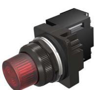
30mm BlackMax, Epoxy Coated Corrosion Resistant Complete Metal Unit Illuminated Indicator Light Full Voltage type, 12V AC/DC Incandescent Lamp, BA9s Glass Lens, Red UL Listed, CSA Certified NEMA 1,3,3R,4,4X,12,13 & Automotive Standards
