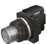
30mm BlackMax, Epoxy Coated Corrosion Resistant Complete Metal Unit Illuminated Indicator Light Full Voltage type, 6V AC/DC LED Lamp, BA9s Glass Lens, Clear UL Listed, CSA Certified NEMA 1,3,3R,4,4X,12,13 & Automotive Standards
