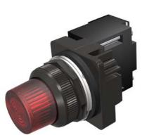
30mm BlackMax, Epoxy Coated Corrosion Resistant Complete Metal Unit Illuminated Indicator Light Full Voltage type, 6V AC/DC Super Bright LED Lamp, BA9s Glass Lens, Red UL Listed, CSA Certified NEMA 1,3,3R,4,4X,12,13 & Automotive Standards
