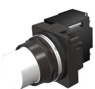
30mm BlackMax, Epoxy Coated Corrosion Resistant Complete Metal Unit Illuminated Indicator Light Transformer type, 480V AC LED Lamp, BA9s Plastic Lens, White UL Listed, CSA Certified NEMA 1,3,3R,4,4X,12,13 & Automotive Standards
