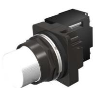
30mm BlackMax, Epoxy Coated Corrosion Resistant Complete Metal Unit Illuminated Indicator Light Transformer type, 120V AC LED Lamp, BA9s Plastic Lens, White UL Listed, CSA Certified NEMA 1,3,3R,4,4X,12,13 & Automotive Standards
