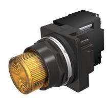
30mm BlackMax, Epoxy Coated Corrosion Resistant Complete Metal Unit Illuminated Indicator Light Full Voltage type, 24V AC/DC Incandescent Lamp, BA9s Plastic Lens, Amber UL Listed, CSA Certified NEMA 1,3,3R,4,4X,12,13 & Automotive Standards
