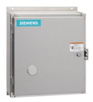
Non-reversing NEMA contactor, Size 4, Three phase full voltage, Contactor amp rating 135A, 3 wire (NO aux included), 380-440/440-480V 50/60Hz coil, Noncombination type, Encl NEMA type 4X 304 S-Steel, Water/dust tight noncorrosive, Extra-wide enclosure
