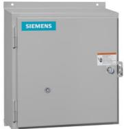
Non-reversing contactor, Size 3 1/2, Three phase full voltage, Contactor amp rating 115A, 3 wire (NO aux included), 110V 50Hz / 120V 60Hz coil, Non-combination type, Encl. NEMA type 4X fiberglass, Water/dust tight noncorrosive, Standard width enclosure
