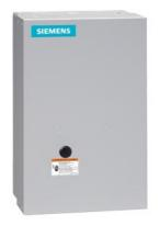
Non-reversing contactor, Size 1 3/4, Three phase full voltage, Contactor amp rating 40A, 3 wire (NO aux included), 240V 50Hz / 277V 60Hz coil, Non-combination type, Enclosure NEMA type 1, Indoor general purpose use, Extra-wide enclosure
