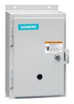
Non-reversing contactor, Size 1 3/4, Three phase full voltage, Contactor amp rating 40A, 3 wire (NO aux included), 190-220/220-240V 50/60Hz coil, Non-combination type, Enclosure NEMA type 12, Dust/drip proof for indoors, Extra-wide enclosure
