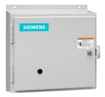
Non-reversing contactor, Size 1 3/4, Three phase full voltage, Contactor amp rating 40A, 3 wire (NO aux included), 240V 50Hz / 277V 60Hz coil, Non-combination type, Enclosure NEMA type 12, Dust/drip proof for indoors, Standard width enclosure
