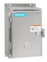
Non-reversing contactor, Size 1 3/4, 4 power poles, Contactor amp rating 40A, 3 wire (NO aux included), 190-220/220-240V 50/60Hz coil, Non-combination type, Encl NEMA type 4X 304 S-Steel, Water/dust tight noncorrosive, Standard width enclosure
