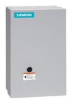
Non-reversing NEMA contactor, Size 1, Three phase full voltage, Contactor amp rating 27A, 3 wire (NO aux included), 380-440/440-480V 50/60Hz coil, Non-combination type, Enclosure NEMA type 1, Indoor general purpose use, Extra-wide enclosure
