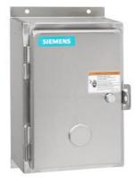
Non-reversing NEMA contactor, Size 1, Single phase full voltage, Contactor amp rating 27A, 3 wire (NO aux included), 190-220/220-240V 50/60Hz coil, Noncombination type, Encl NEMA type 4X 304 S-Steel, Water/dust tight noncorrosive, Standard width enclosure
