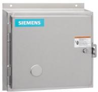
Non-reversing NEMA contactor, Size 0, Three phase full voltage, Contactor amp rating 18A, 3 wire (NO aux included), 240V 50Hz / 277V 60Hz coil, Noncombination type, Encl NEMA type 4X 304 S-Steel, Water/dust tight noncorrosive, Extra-wide enclosure
