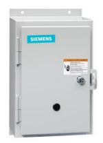
Non-reversing NEMA contactor, Size 0, Three phase full voltage, Contactor amp rating 18A, 3 wire (NO aux included), 220-240/440-480VAC 60Hz coil, Non-combination type, Enclosure NEMA type 12, Dust/drip proof for indoors, Extra-wide enclosure
