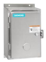
Non-reversing NEMA contactor, Size 0, Three phase full voltage, Contactor amp rating 18A, 3 wire (NO aux included), 24VAC 50-60Hz coil, Non-combination type, Encl NEMA type 4X 304 S-Steel, Water/dust tight noncorrosive, Standard width enclosure
