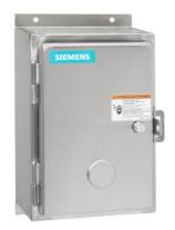
Non-reversing NEMA contactor, Size 0, Three phase full voltage, Contactor amp rating 18A, 3 wire (NO aux included), 190-220/220-240V 50/60Hz coil, Non-combination type, Encl NEMA type 4X 304 S-Steel, Water/dust tight noncorrosive, Standard width enclosure
