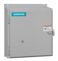
Non-reversing NEMA contactor, Size 0, Three phase full voltage, Contactor amp rating 18A, 3 wire (NO aux included), 110V 50Hz / 120V 60Hz coil, Non-combination type, Encl. NEMA type 4X fiberglass, Water/dust tight noncorrosive, Standard width enclosure
