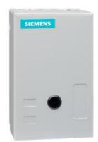
Non-reversing NEMA contactor, Size 0, Three phase full voltage, Contactor amp rating 18A, 3 wire (NO aux included), 190-220/220-240V 50/60Hz coil, Non-combination type, Enclosure NEMA type 1, Indoor general purpose use, Standard width enclosure
