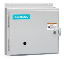
Non-reversing NEMA contactor, Size 0, Three phase full voltage, Contactor amp rating 18A, 3 wire (NO aux included), 208VAC 60Hz coil, Non-combination type, Enclosure NEMA type 12, Dust/drip proof for indoors, Standard width enclosure
