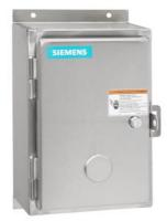
Non-reversing NEMA contactor, Size 0, 4 power poles, Contactor amp rating 18A, 3 wire (NO aux included), 240V 50Hz / 277V 60Hz coil, Non-combination type, Encl NEMA type 4X 304 S-Steel, Water/dust tight noncorrosive, Standard width enclosure
