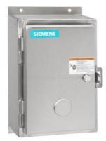
Non-reversing NEMA contactor, Size 0, 4 power poles, Contactor amp rating 18A, 3 wire (NO aux included), 380-440/440-480V 50/60Hz coil, Non-combination type, Encl NEMA type 4X 304 S-Steel, Water/dust tight noncorrosive, Standard width enclosure
