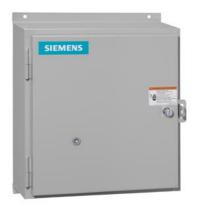
Non-reversing NEMA contactor, Size 0, 4 power poles, Contactor amp rating 18A, 3 wire (NO aux included), 24VAC 50-60Hz coil, Non-combination type, Encl. NEMA type 4X fiberglass, Water/dust tight noncorrosive, Standard width enclosure
