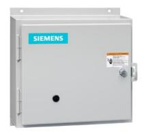
Non-reversing NEMA contactor, Size 0, 4 power poles, Contactor amp rating 18A, 3 wire (NO aux included), 220-240/440-480VAC 60Hz coil, Non-combination type, Enclosure NEMA type 12, Dust/drip proof for indoors, Standard width enclosure
