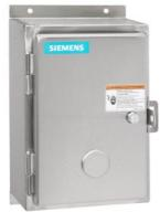
Non-reversing NEMA contactor, Size 0, Single phase full voltage, Contactor amp rating 18A, 3 wire (NO aux included), 110V 50Hz / 120V 60Hz coil, Noncombination type, Encl NEMA type 4X 304 S-Steel, Water/dust tight noncorrosive, Standard width enclosure
