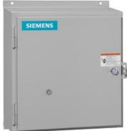
Non-reversing NEMA contactor, Size 0, Single phase full voltage, Contactor amp rating 18A, 3 wire (NO aux included), 220-240/440-480VAC 60Hz coil, Noncombination type, Encl. NEMA type 4X fiberglass, Water/dust tight noncorrosive, Standard width enclosure
