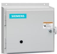
Non-reversing NEMA contactor, Size 0, Single phase full voltage, Contactor amp rating 18A, 3 wire (NO aux included), 24VAC 50-60Hz coil, Non-combination type, Enclosure NEMA type 12, Dust/drip proof for indoors, Standard width enclosure
