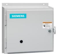
Non-reversing NEMA contactor, Size 0, Single phase full voltage, Contactor amp rating 18A, 3 wire (NO aux included), 110V 50Hz / 120V 60Hz coil, Non-combination type, Enclosure NEMA type 12, Dust/drip proof for indoors, Standard width enclosure
