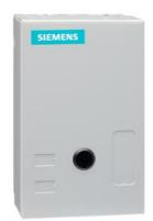
Non-reversing NEMA contactor, Size 00, Single phase full voltage, Contactor amp rating 9A, 3 wire (NO aux included), 190-220/220-240V 50/60Hz coil, Noncombination type, Enclosure NEMA type 1, Indoor general purpose use, Standard width enclosure
