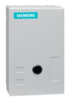
Non-reversing NEMA contactor, Size 00, Single phase full voltage, Contactor amprating 9A, 3 wire (NO aux included), 110V 50Hz / 120V 60Hz coil, Non-combination type, Enclosure NEMA type 1, Indoor general purpose use, Standard width enclosure
