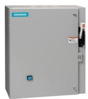
2-speed 3-phase motor starter, Size 1, One winding consequent pole, Constant or variable torque, Solid-state overload relays, Low Spd OLR range 3-12A, High Spd OLR range 5.5-22A, 110V 50Hz / 120V 60Hz coil, Combination type, 25A circuit breaker, Enclosure NEMA type 4/12, Water/dust tight for outdoors
