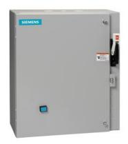
2-Speed 3-phase motor starter Size 1 Two separate windings Constant or variable torque Solid-state overload relays Low SPD OLR range 3-12A High SPD OLR range 5.5-22A 110V 50HZ / 120V 60HZ coil Combination type 30Amp disconnect switch Enclosure NEMA type 4/12 Water/dust tight for outdoors
