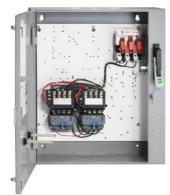
2-speed 3-phase motor starter, Size 1, One winding consequent pole, Constant or variable torque, Solid-state overload relays, Low Spd OLR range 0.75-3.4A, High Spd OLR range 5.5-22A, 110V 50Hz / 120V 60Hz coil, Combination type, 30A disconnect switch, Enclosure NEMA type 4/12, Water/dust tight for outdoors
