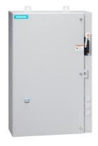
2-speed 3-phase motor starter Size 0 Two separate windings Constant or variable torque Solid-state overload relays Low SPD OLR range 3-12A High SPD OLR range 5.5-22A 110V 50HZ / 120V 60HZ coil Combination type 30Amp disconnect switch Encl NEMA type 4X 304 S-steel Water/dust tight noncorrosive
