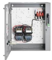
2-speed 3-phase motor starter, Size 0, One winding consequent pole, Constant or variable torque, Solid-state overload relays, Low Spd OLR range 3-12A, High Spd OLR range 5.5-22A, 110V 50Hz / 120V 60Hz coil, Combination type, 30A disconnect switch, Enclosure NEMA type 4/12, Water/dust tight for outdoors
