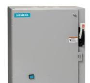
2-speed 3-phase motor starter Size 0 Two separate windings Constant or variable torque Solid-state overload relays Low SPD OLR range 3-12A High SPD OLR range 5.5-22A 110-120/220-240VAC 60HZ coil Combination type 30Amp disconnect switch Enclosure NEMA type 4/12 Water/dust tight for outdoors
