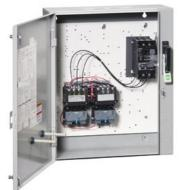
2-speed 3-phase motor starter Size 0 Two separate windings Constant horsepower Solid-state overload relays Low SPD OLR range 3-12A High SPD OLR range 5.5-22A 110V 50HZ / 120V 60HZ coil Combination type 25Amp circuit breaker Enclosure NEMA type 4/12 Water/dust tight for outdoors
