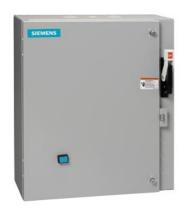
2-speed 3-phase motor starter Size 0 One winding consequent pole Constant or variable torque Solid-state overload relays Low SPD OLR range 0.25-1A High SPD OLR range 0.75-3.4A 110V 50HZ / 120V 60HZ coil Combination type 3Amp circuit breaker Enclosure NEMA type 1 Indoor general purpose use
