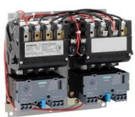
2-speed 3-phase motor starter Size 2 1/2 Two separate windings Constant or variable torque Solid-state overload relays Low SPD OLR range 13-52a High SPD OLR range 25-100A 110V 50HZ / 120V 60HZ coil Enclosure NEMA type (open) No enclosure
